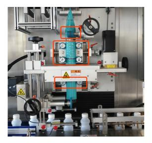
(2) New two belts system to keep running on conveyor
